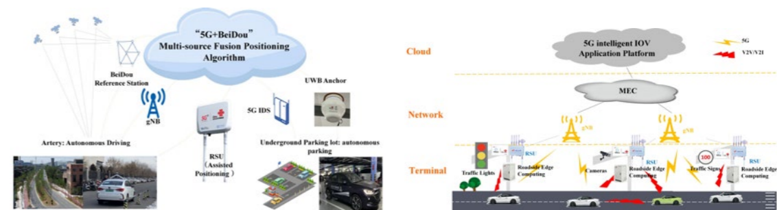
● “5G+Beidou” Multi-source Fusion High-precision Positioning & 5G+C-V2X integrated networking
