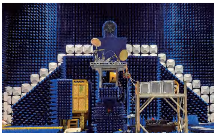
卫星通信载荷无线对接测试 Wireless Interface Test Solution for Satellite Communication Payloads
