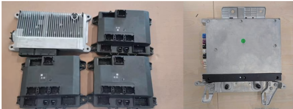
左图区域控制器，右图中央计算平台 The left image shows the VIU (Vehicle Infranet Unit); the right image shows the OIB (One Intelligent Brain)
