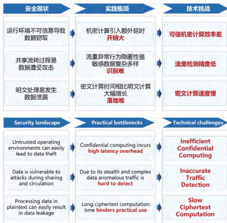
面向云系统的数据安全防护三个技术难题 Three Technical Bottlenecks Facing Data Security Protection in Cloud Systems
