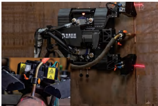
无轨导全位置爬行焊接机器人 - 激光扫描 Track-Free All-Position Crawling Welding Robot - Laser Scanning
