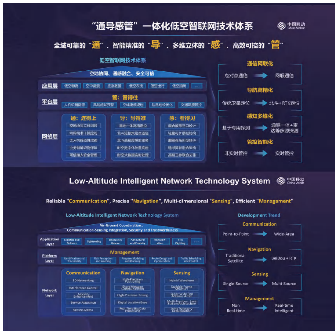
“通导感管”一体化低空智联网技术体系 An Integrated "Communication, Navigation, Sensing and Management" Low-Altitude Intelligent Network Technological System
