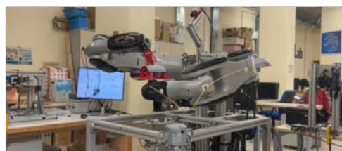
▲ Hands-on platform that displays collaborative tasks between robots for use in using FBG photonics to press indented sensing skin
